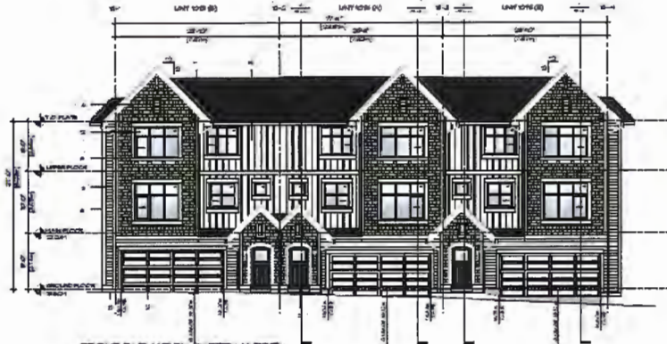
1 FRONT ELEVATION (NORTH-WEST) SCALE 1/8"=1'-0"
