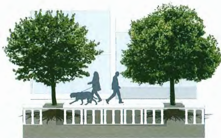
Figure 39: Provide soil cells to allow for healthy long-term growth.
