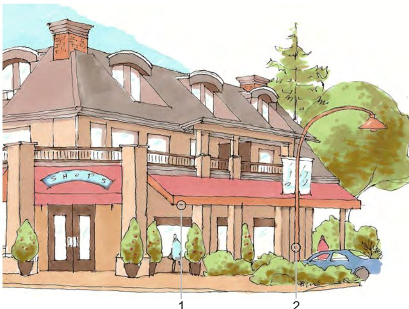
**Figure 30. Continuous overhangs**
