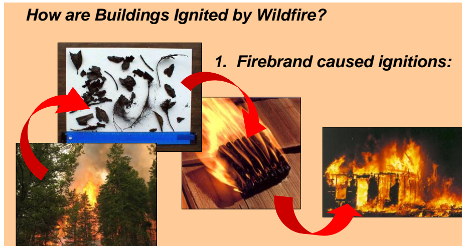
Figure 15. Firebrand caused ignitions: burning embers are carried ahead of the fire front and alight on vulnerable building surfaces.
